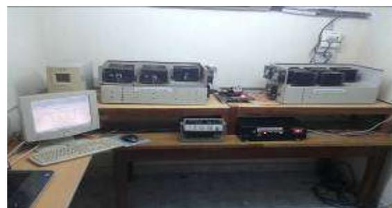
**Electronic Load Bank and Instrumentation setup**
